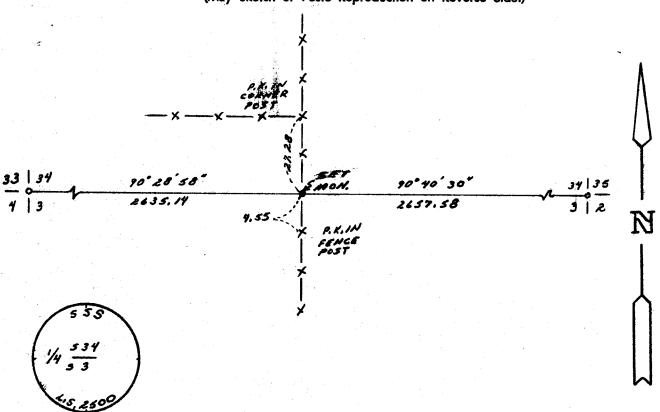
John A. Steil certify that I have carefully performed or reviewed the work done on the diagrammed corner as reported on this recordation form and approve the L.S. 2500
